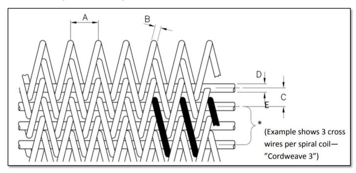
**NOTE:** When measuring pitch, it is best practice to measure over 10 pitches and divide by 10 to obtain the average pitch.
