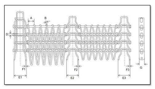
**NOTE:** When measuring pitches A & C, it is best practice to measure over 10 pitches and divide by 10 to obtain the average pitch.
