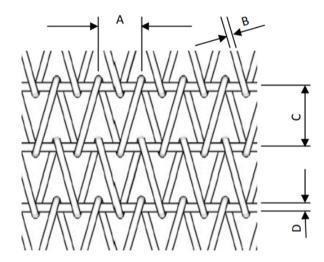
**NOTE:** When measuring pitches A & C, it is best practice to measure over 10 pitches and then divide by 10 to obtain the average pitch.
