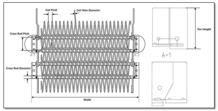
**NOTE:** When measuring Coil Pitch, it is best practice to measure over 10 pitches and then divide by 10 to obtain the average pitch.
